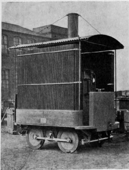
Fig. 22—Loftus Perkins high-pressure tram locomotive by Greenwood and Batley, Ltd., 1878
