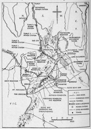
When complete, the entire scheme will provide nearly 2,000,000 acre feet of water annually in the Murray and Murrumbidgee, which will allow about 1000 square miles to be cultivated at an annual turnover of £30,000,000. The installed capacity will be about 2500MW overall, and the annual energy output 5500 × 10°kWh, i.e. an overall load factor of about 25 per cent. The total cost of the scheme is estimated at about £375 million. Its power stations are listed in the table herewith.
